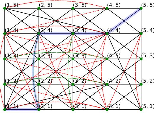
Joint State Graph for a 5node environment graph. Red (green) edges represent traversing risk edge without (with) support.
